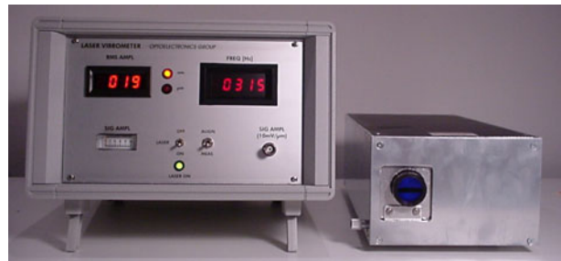
Figure 10. Photograph of prototype self-mixing LD vibrometer. Left, electronic unit; right, optical head.
