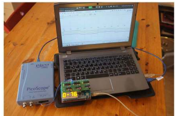
Fig 9. Experimental setup, sketch and photograph. Two DPLLs coupled through a microcontroller, which artificially introduces a transmission delay. An oscilloscope samples the periodic signals of the DPLLs. © 2015 IEEE. Reprinted, with permission, from IEEE Proceedings: Synchronization of mutually coupled digital PLLs in massive MIMO systems .
