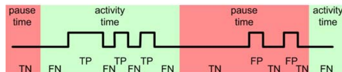
Figure 5. Definition of TP, FP, TN, FN during activity and pause time.
