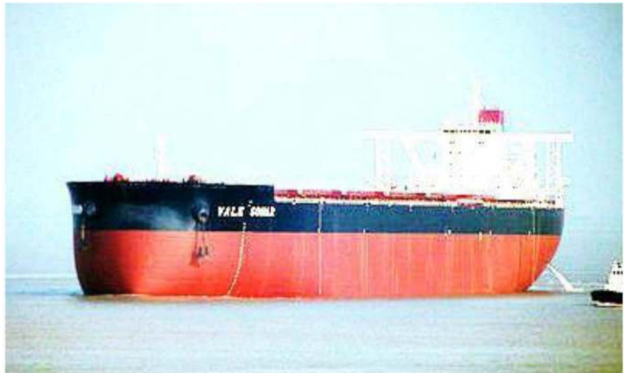
Figure 10. A Vale ship called “Valemax” or VLOC (very large ore carrier). Source: Goulielmos [24].
