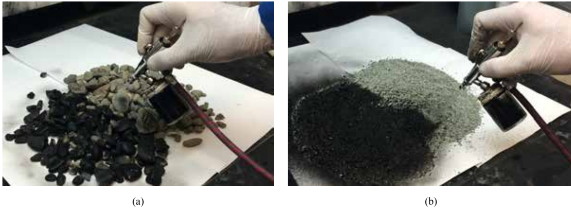
Figure 3. MWNT-latex inks are airbrushed to form thin films on (a) large or coarse aggregates and (b) sand.
