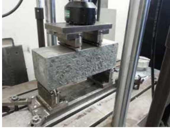
Figure 5. A simply-supported beam specimen is mounted in an MTS load frame for four-point bending testing based on the guidelines specified in ASTM C78.
