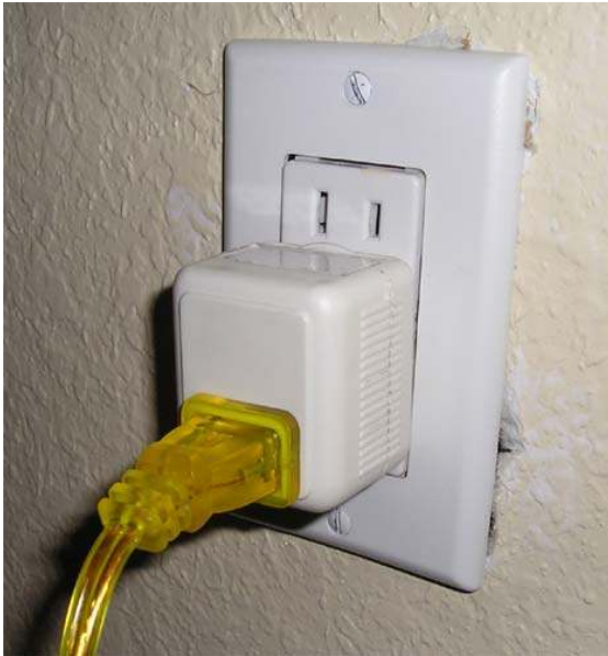
Figure 26. The smart plug used in the Gator Tech Smart House.
