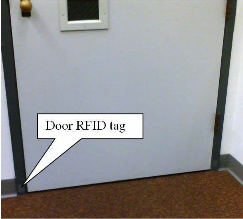
Figure 10. RFID tag describing a door
