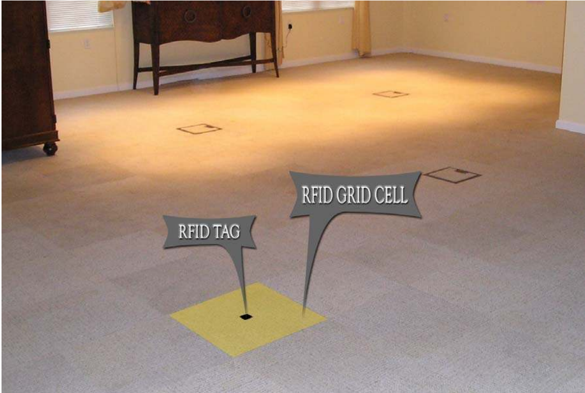
Figure 12. RFID grid in the GTSH
