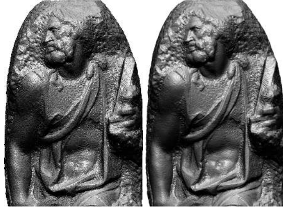
Figure 6: Rendering of the original (left) and decompressed Stanford St Matthew (right), both have 93.4 million points. R = 3mm, N_{bins} = 16
