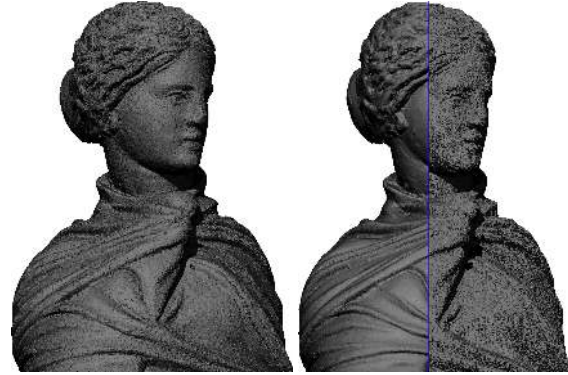
Figure 8: Comparison with kd-tree based coding. Left : original point cloud. Right : comparative decompression. Even with more bits per point (4.83 against 0.6 in our method), the right part encoded with [GD02] is less accurate than our approach (left part). R = 0.7\text{mm} , N_{bins} = 16
