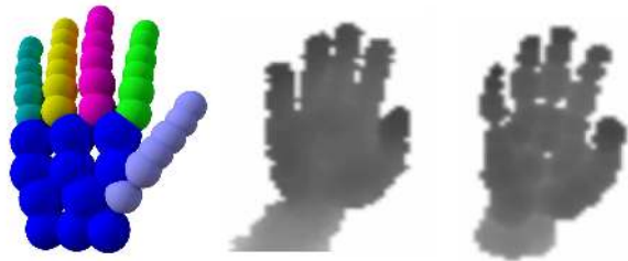
Figure 2. Hand model used during model fitting. Left: Our hand model approximation with 41 spheres; Middle: Real depth map; Right: Rendered depth map from differentiable ray-tracing.
