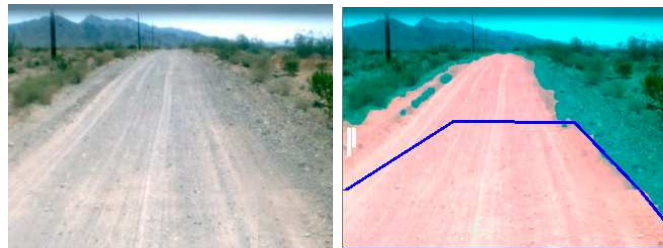
Fig. 3. Input raw image (left) and output data of the computer vision part of the algorithm. The right image duplicates the left, overlaying the training data from the laser map (blue polygon), and the pixels identified as drivable (red area). The scene is the same as in Fig. 2.
