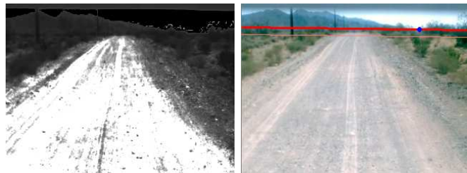
Fig. 4. Intermediate processing steps: The left image shows the similarity of each pixel to our road model (before thresholding). The right image shows the border between ground and sky, as found by the algorithm.
