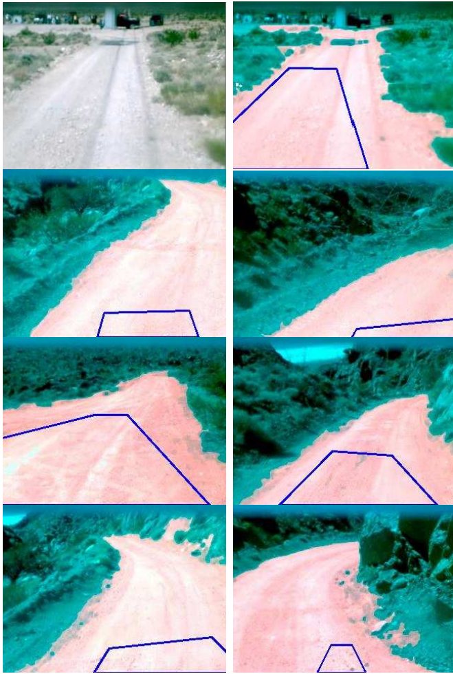
Fig. 10. Scenes of the 2005 Grand Challenge: The first row shows a media watch point, with the raw camera image on the left and the classification result on the right. The next rows show classification results during traversal of the mountainous Beer Bottle Pass. The blue training area varies significantly because the rugged nature of the environment causes Stanley to shake more, which in turn sometimes leaves holes in the laser map. The module that fits an area-maximized training quadrangle into this map is conservative and tries not to cover these holes. A training area that varies from frame to frame however does not harm segmentation performance, since the algorithm is executed at high frame rate and learns a road model that incorporates history.
