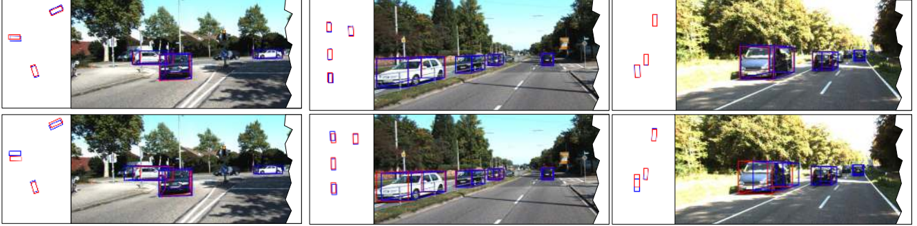
Figure 4. Visualization of Bird’s View Box and 3D Bounding Box. Our results (top row) and results from GeoNet [33] (bottom row) are presented. The ground truth is in red while the prediction is in blue. Our predictions have a larger overlapping with the ground truth box.
