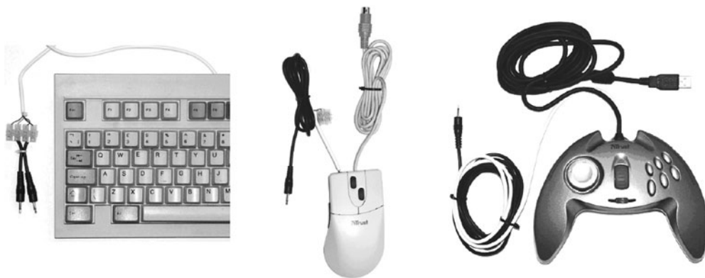
Figure 3. Typical response devices with active switch closure flying leads soldered to their primary and/or secondary buttons so that they can be controlled from the Black Box Toolkit.
