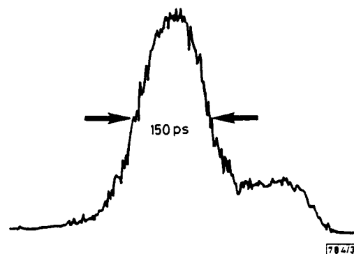
Fig. 3 Pulse output from 14 m modelocked fibre laser
