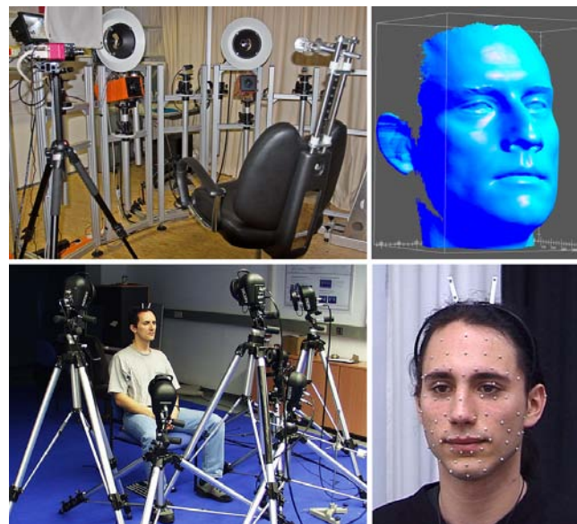
Figure 2: ABW Scanner (top left) and face scan example (top right); Motion Capture system (lower left) and reflective marker setup with additional head tracking target (lower right).
