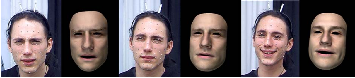
Figure 1: Three examples of facial expressions retargeted from Motion Capture onto a morphable 3D face model (from left to right: Confusion , Thinking , Pleasant Surprise ).
