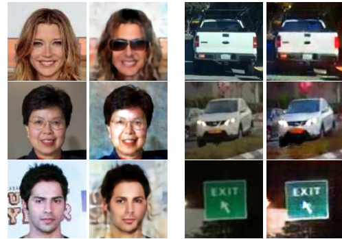
Figure 1. Examples of semantic adversarial attacks with a single modifiable attribute. The first and third columns are original images. Semantic adversarial examples (Columns 2 and 4) are generated by optimizing over the manifold of parametric (attribute) generative models to fool deep classifiers; specifically for adversarial facial attributes for Col. 2 and illumination for Col. 4.
