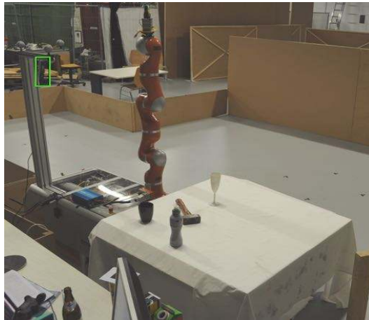
Figure 12: The table is in front of the mobile platform. The range sensor is marked by the green rectangle.
