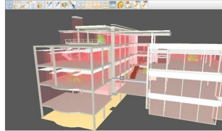
Fig. 5. Structural view of a building. This view is required for structure engineers. The corresponding graph provides all elements needed to make structure calculations.
