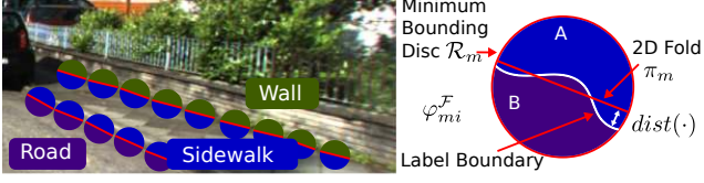
Figure 4: Geometric Unary Potentials. Left: We encourage label changes at 3D curbs or folds after projection into the image domain. Right: This constraint ( \varphi_{mi}^{\mathcal{F}} ) is implemented by pixel unary potentials inside each minimum bounding disc \mathcal{R}_m around each 2D curb or fold segment m .
