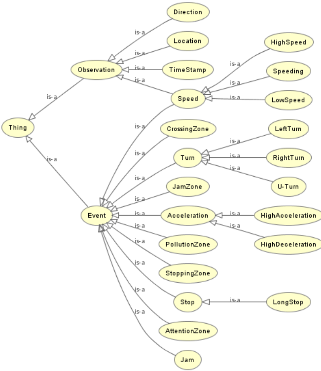
Fig. 4. Static knowledge as a high-level ontology (Properties are not included in this figure).
