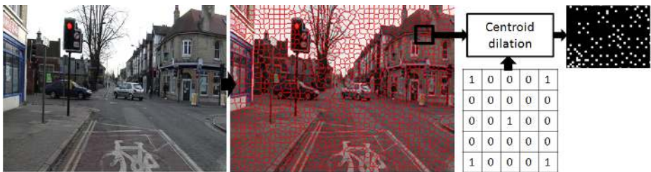
Fig. 3. The number of training samples is sub-sampled to reduce the computational training overhead. The incoming image is over-segmented using superpixels. Then, patches centered at the centroid of each superpixel and several pixels in its surrounding area are selected as training samples.
