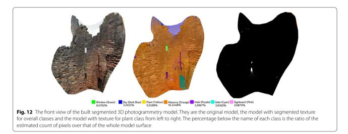
algorithm that is capable of handling segmentation tasks in complex scenarios. It is further combined with photogrammetry to automatically process the crowdsourced photographs. This can significantly save human and capital resources spent on on-site inspection and management of remote built heritage sites.
