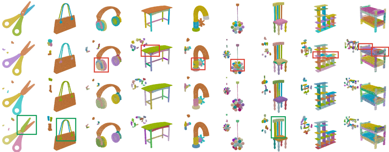
Fig. 6 Visual comparison of part instance segmentation on the test set of PartNet. Part instances at the fine level are colored with random colors. 1st row: part instance ground-truth. 2nd row: results of our multi-level baseline † . 3rd row: results of our cross-level fusion † without using semantic region centers. 4th row: results of our cross-level fusion using semantic region centers. The corresponding shifted points are rendered at the top left of each instance segmentation image. Green and red boxes represent good and bad instances, respectively.
