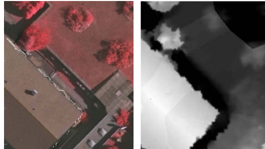
Figure 8: Zoomed in image of the bottom left corner of the image in Figure 3, where the vegetation area was misclassified as a building in all three models. The RGB image on the left and the normalized DSM on the right.
