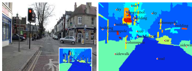
Figure 1. Semantic segmentation of a street sequence. Left: An input image with ground-truth in-set. Right: Output of the proposed method.
