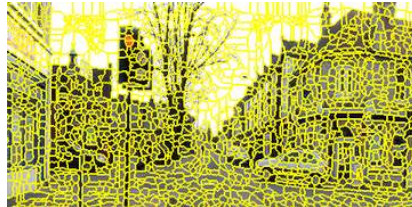
Figure 4. The watershed LoG based superpixels shown on a part of the image from Fig. 1.
