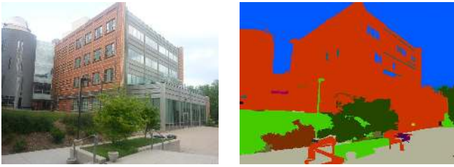
Fig. 1. Semantic Segmentation. Left: original image; Right: color coded semantic categories. Detected man-made structure are colored red.
