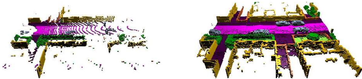
Figure 5: Left: Visualization of the incomplete input for the semantic scene completion benchmark. Note that we show the labels only for better visualization, but the real input is a single raw voxel grid without any labels. Right: Corresponding target output representing the completed and fully labeled 3D scene.
