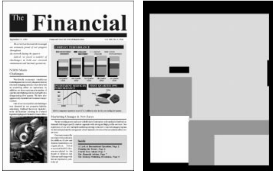
Figure 2: One sample image and its classification result image. The error rate is 3.64%. White: photograph, light gray: graph, dark gray: text, black: background.
