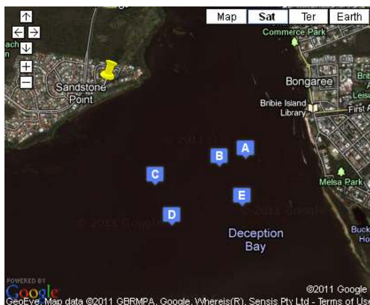
Figure 7. Locations of the SEMAT Mk2 buoys within Deception Bay. Each buoy was labelled A, B, C, D and E respectively. All buoys were identical except for Node A, which contained an above water light sensor. The base station was located on Sandstone Point (indicated by the yellow pin). The buoy ranges from the base station were as follows: Node A—1.4 km, Node B—1.3 km, Node C—1.0 km, Node D—1.4 km and Node E—1.7 km.
