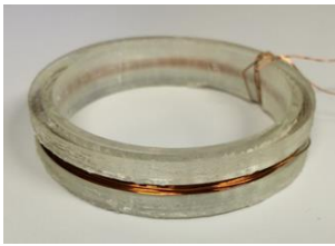
Fig. 5 50-turn enameled copper coil, with conductor radius 0.15 mm, cover thickness 0.03 mm. The coil is wound around a bobbin, made by a photocurable 3D printer, whose radius is 30 mm.
