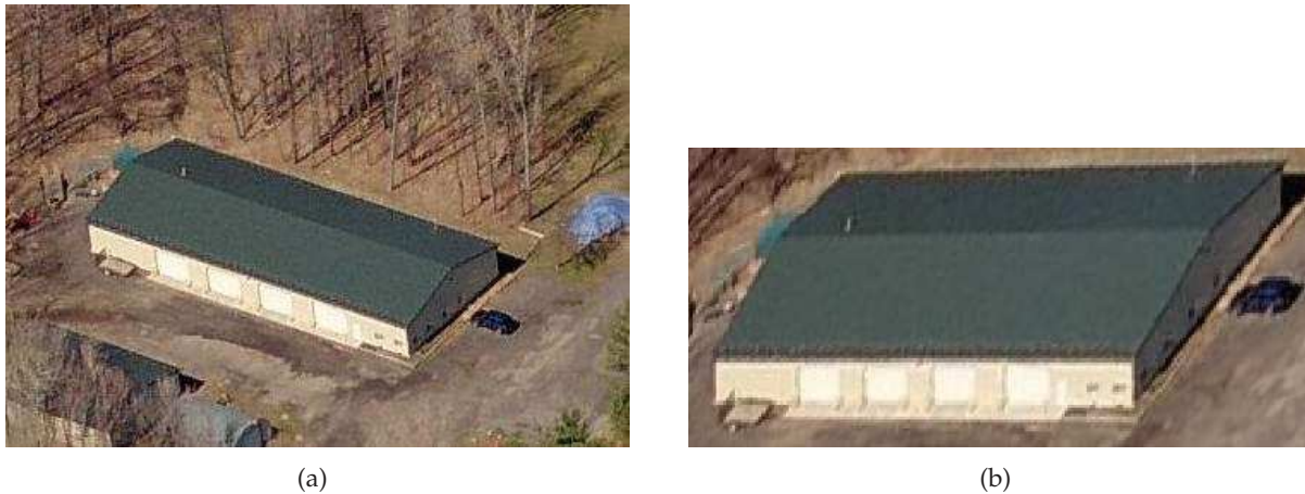
Figure 5.27: Material map for shed model. (a) original frame array image (b) re-projected view used to generate material map for one facet (building side).
