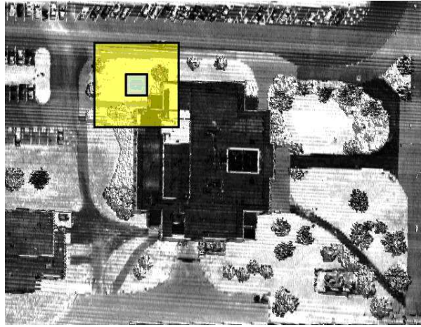
Figure 4.6: Illustration of the Modified Minimum Filter at a single location; minimum height value is calculated in smaller window, points 3m above minimum in larger window are flagged as non-ground points.
