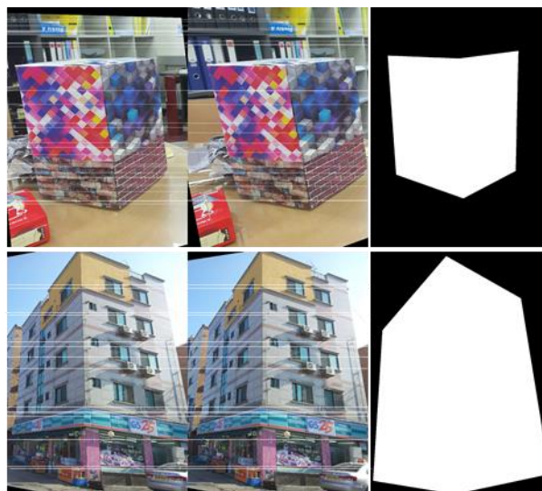
Figure 6. Epipolar resampled stereo images and ROI
