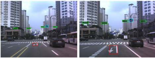
FIGURE 8. Extension to bounding box annotation. In the left figure, bounding boxes of traffic landmarks are manually annotated. The 3D locations of corner points of the bounding boxes can be obtained based on the aligned HD map. The 3D bounding boxes can be propagated to the following frames as an example is shown in the right figure.
