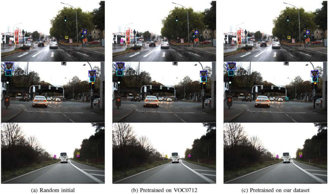
FIGURE 6. Qualitative results on GTSDB varying pretrained dataset. Mandatory, prohibition, danger, and other signs are marked with cyan, magenta, yellow, and blue bounding boxes, respectively. Although the network pretrained on our dataset detects traffic landmarks with reference points, it is more effective than the network pretrained on VOC0712 finetuned to detect German traffic signs using bounding boxes.
