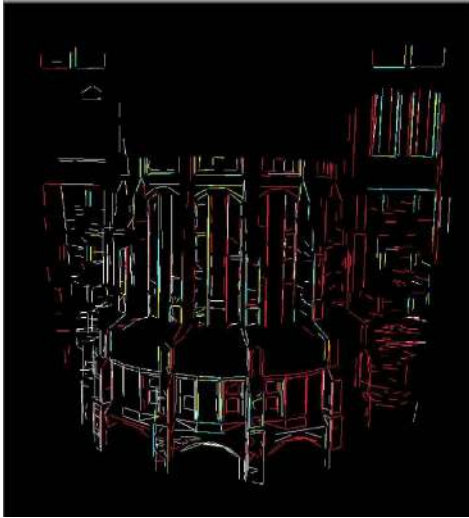
Figure 8. Matching lines between two scans. White/red lines are border lines, and yellow/blue lines are the matching lines from two images respectively.
