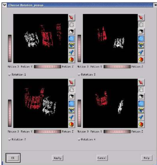
Figure 6. A set of possible orientations between the two coordinate systems is presented to the user to choose from. In this example the rotation in the upper left corner corresponds to the correct result.
