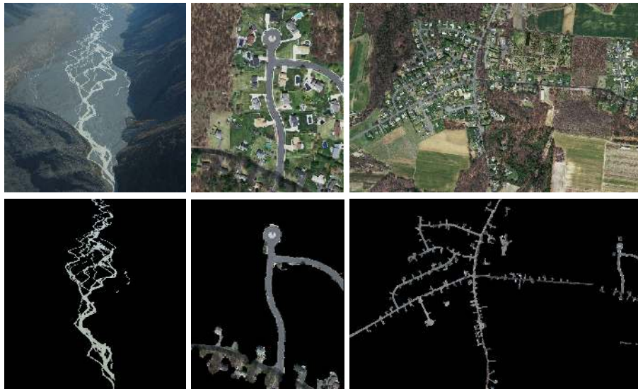
Fig. 6: Segmentation of river and road from aerial images. Left: segmentation of the Murchison river. Middle and right: segmentation of road from aerial images (the images are borrowed from Massachusetts Roads Dataset [31]).
