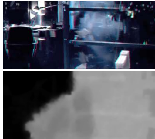
Figure 7. Depth Failure in “Batman - The Dark Knight”. Due to an abrupt change of scenery during the shot, the disparity map lost its continuity and a flat map is obtained. (top) original frame. (bottom) disparity map.
