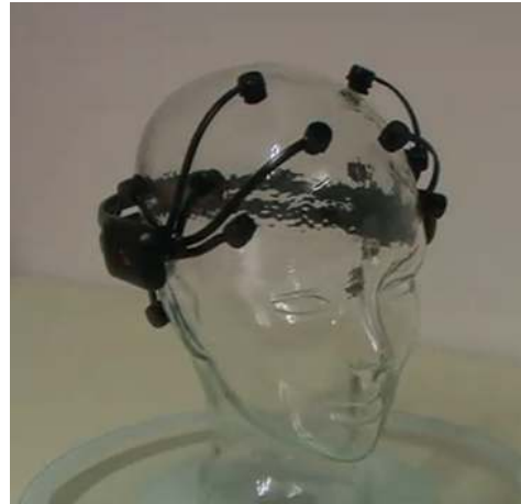
Fig. 4. Epoc neuroheadset from Emotive. The cap is connected wirelessly to the computer.
