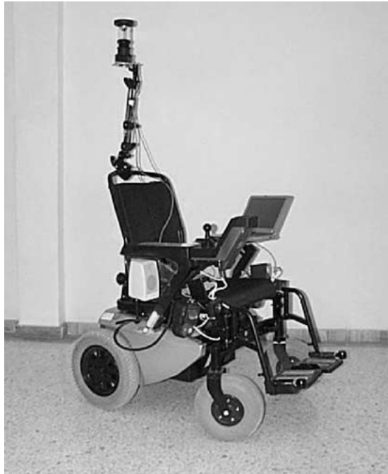
Figure 7. Side view of the developed experimental robotic wheelchair prototype.
