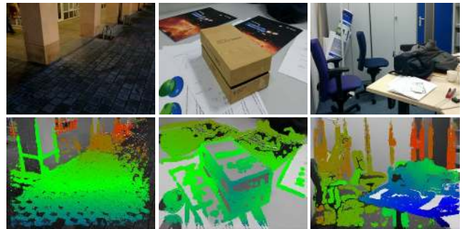
Figure 3: Examples of semi-dense depth maps estimated in real-time on a smartphone. See also the attached video.
