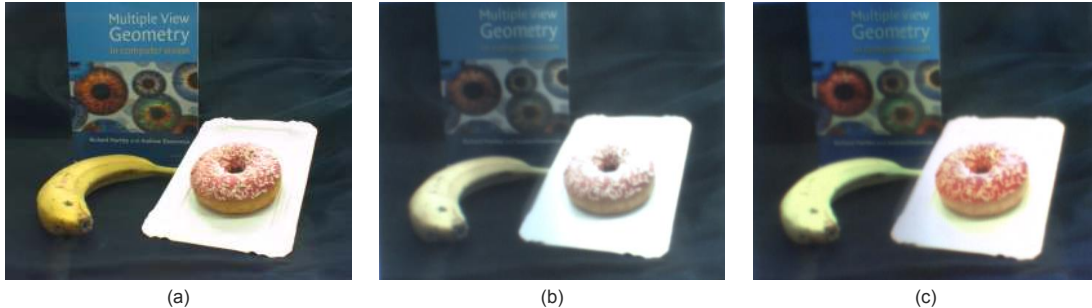
Fig. 1. A demonstration of the color reproduction problem in OST-HMDs and a result of our correction method. (a) A physical scene captured by a user-perspective camera. (b) A captured image of (a) rendered on a consumer OST-HMD with an opaque background. (c) A captured image of a pre-processed image of (a) displayed on the HMD. Rendering (a) on the display causes chromatically distorted image (b), which is undesirable for natural AR experiences. The corrected image (c) reproduces the original color better, thus potentially provides better color constancy in visual-processing AR applications.
