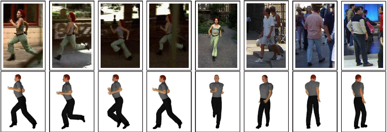
Figure 5. Qualitative 3D reconstruction results obtained on images from the movie ‘Run Lola Run’ (block of leftmost 5 images) and the INRIA pedestrian dataset (rightmost 3 images) [8]. (a) Top row shows the original images, (b) Bottom row shows automatic 3D reconstructions.
