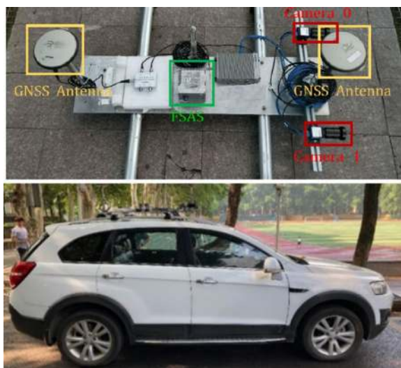
Fig. 4 The experimental equipment including the hardware platform (top) and the data acquisition vehicle (bottom)
