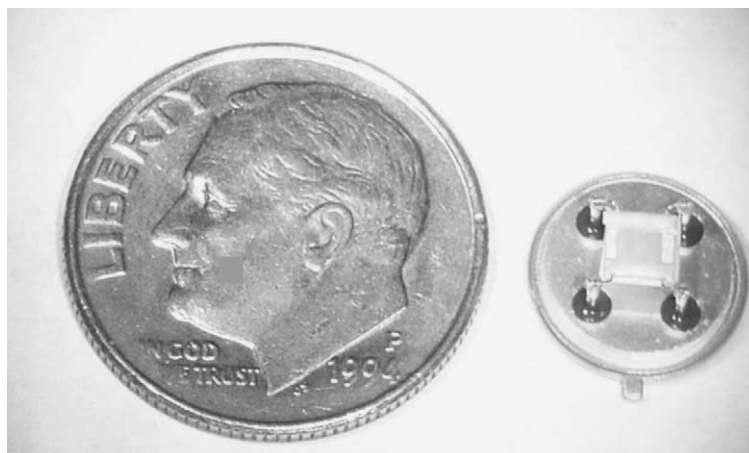
Fig. 1. An UST sensor platform suspended by leads to a TO-8 case. The dime (18 mm diameter) shows the relative size of the sensor and case.
