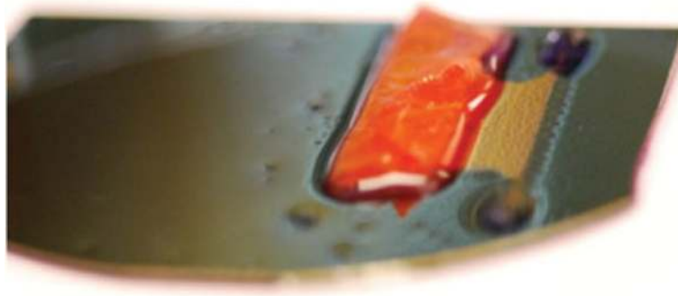
Figure 10. Cyborg cardiac tissue (red) in which a three-dimensional nanowire field-effect transistor network is seamlessly integrated with three-dimensional cultured cardiomyocytes. The width and thickness of the cyborg tissue are ca. 2.5 cm and 1 mm, respectively.
