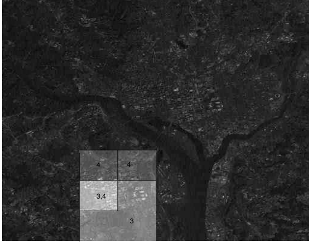
Fig. 5. Illustration of tamper localization by hierarchical semi fragile watermark when image is JPEG compressed with Q=40.
