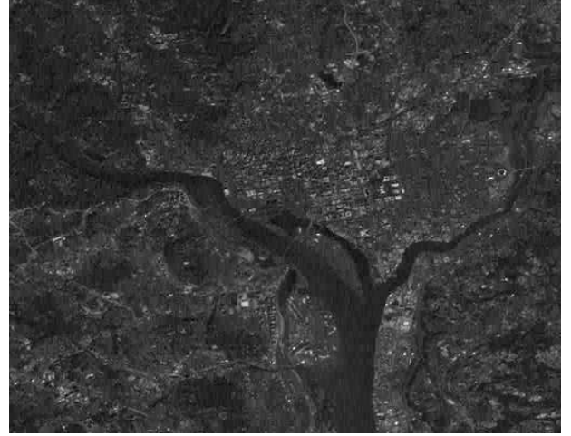
Fig. 3. Watermarked Washsat image. ( P_0 = 30, P_1 = 3, Q=30, L=4, R=2 and \gamma=1 . PSNR=30.53 dB)
