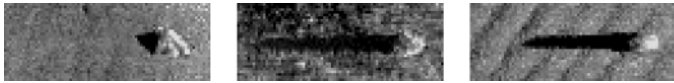
Fig. 5. These positive MLO examples have varying shadow lengths, but an approximately consistent highlight location within the window.
