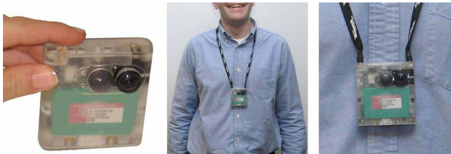
Fig. 1. The SenseCam v2.3 prototype shown standalone and as typically worn by a user. The model pictured here has a clear plastic case which reveals some of the internal components.
