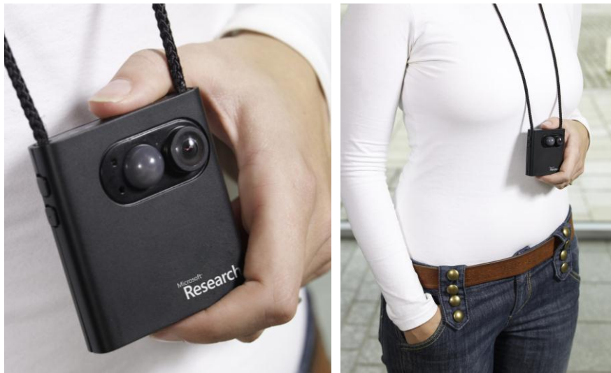
Fig. 1. The SenseCam shown close-up and as typically worn, using an adjustable lanyard. The two side buttons are visible on the left, and there is an additional on-off button on the top of the device. There are three LED lights to indicate various aspects of operation.
