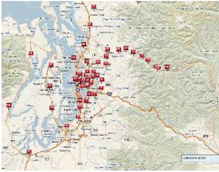
Fig. 1. A 1500 mile path over which we measured UHF spectrum at 57 different locations. The push pins indicate points of measurement.
