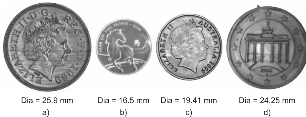
FIG. 9. (a) Image of the obverse of a British two-pence coin, obtained via voltage sensing with LFI using a 2.6 THz QCL, where the beam was modulated by an optical chopper. 60 Reproduced with permission from Dean et al. , Opt. Lett. 36 (13), 2587–2589 (2011). Copyright 2011 OSA Publishing. (b) Image of the reverse of a Lunar Year of the Horse 2014 Gold Coin, obtained via voltage sensing with LFI using a 2.9 THz QCL operating in the pulsed mode. 31 Adapted with permission from Appl. Phys. Lett. 107 (1), 011107 (2015). Copyright 2015 AIP Publishing. (c) Amplitude image of the obverse of an Australian five cent coin obtained via swept-frequency LFI using a 2.59 THz QCL. (d) Amplitude contrast image of the reverse of a German 50 cent coin, imaged over 4 s using a scanning mirror, obtained via voltage sensing with LFI using a 3.3 THz QCL, with triangular current modulation. 92 Adapted with permission from Appl. Phys. Lett. 109 (1), 011102 (2016). Copyright 2016 AIP Publishing.
