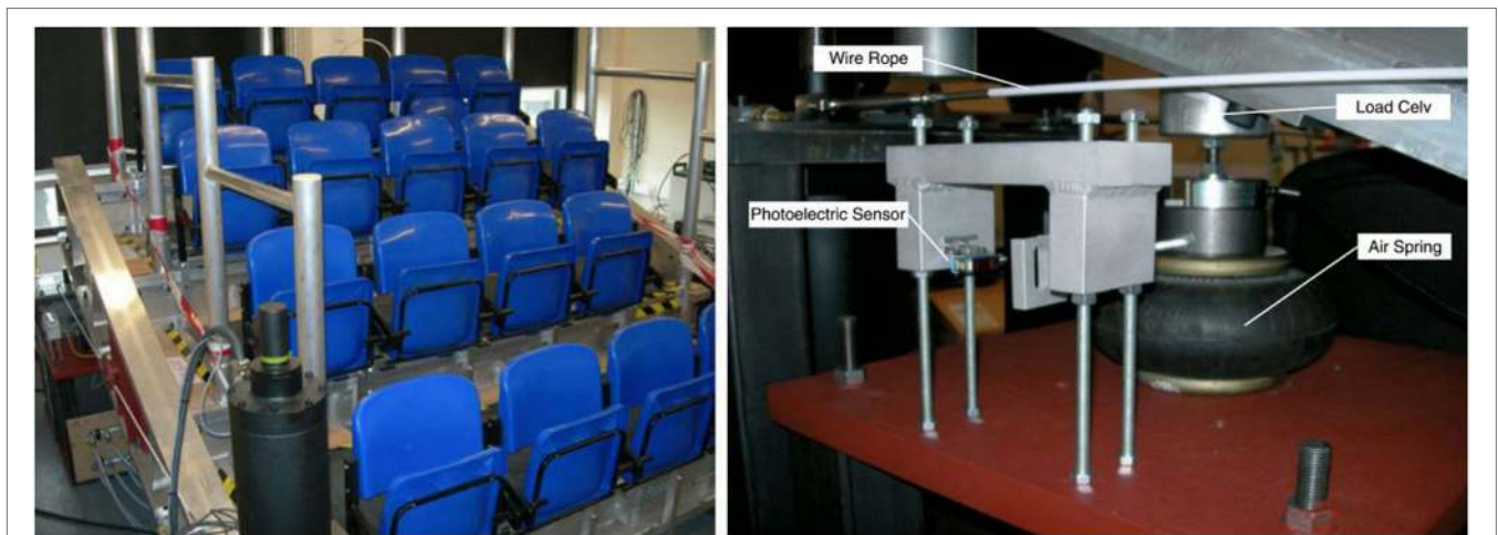
FIGURE 2 | The grandstand rig and the air spring assembly. Reprinted from (Comer et al., 2010) with permission from Springer.
