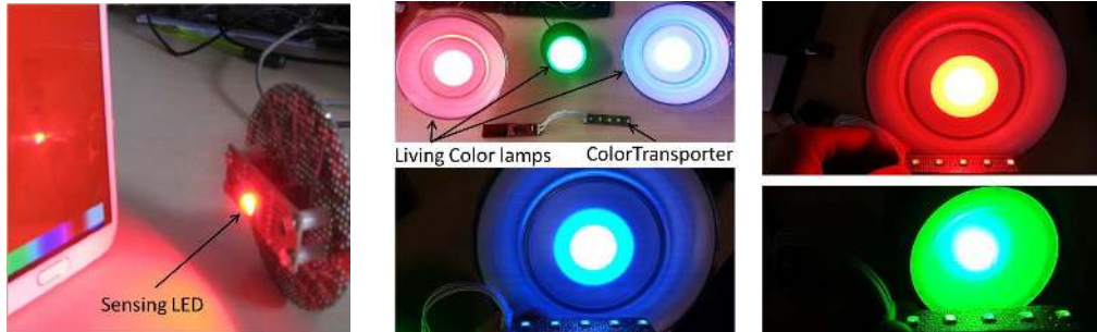
(a) Color sensing LED luminaire adapts its color to the screen of a smart phone.
